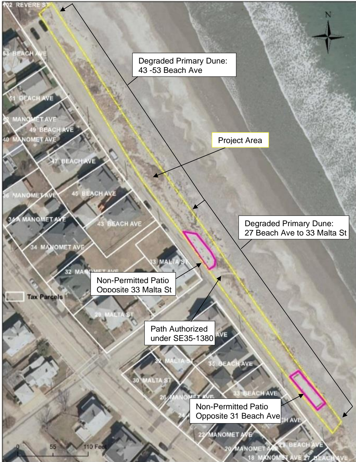
Figure B-1. Google earth aerial showing the ~800 ft section of degraded dune area (yellow) adjacent to 27-53 Beach Ave and the two gaps in the dune at 31-37 Beach Ave and 33 Malta St (pink).
