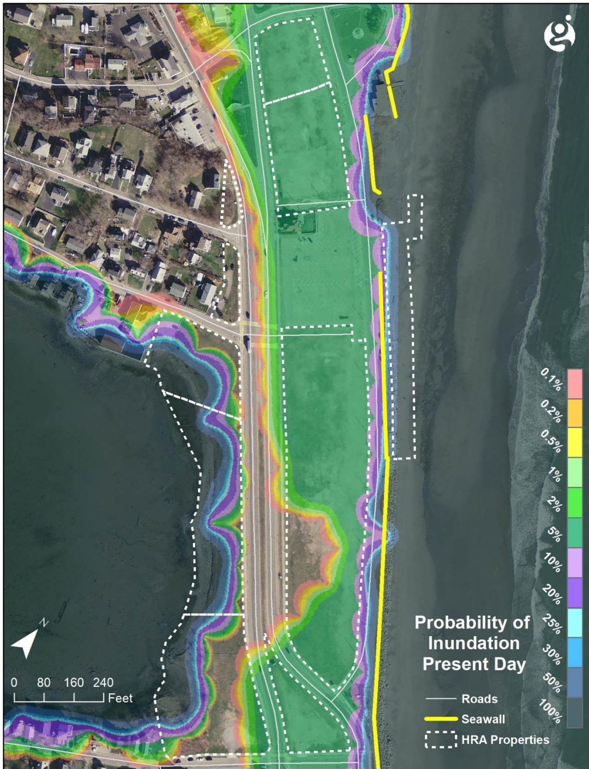
Figure 5. Annual percent chance (probability) of flooding (inundation) for present day conditions using the BH-FRM results for the HRA properties (white outline). Results only valid for HRA properties.
