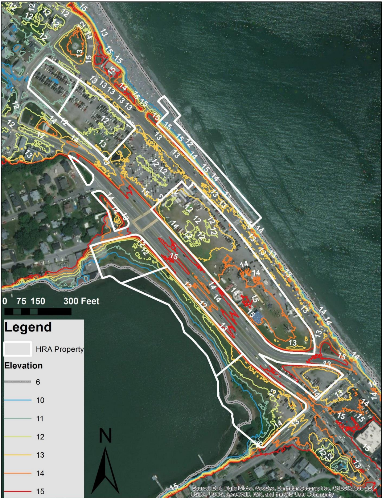
Figure 2. Topographic (elevation) map with 1-foot contours for the HRA Properties (checker board outline).
