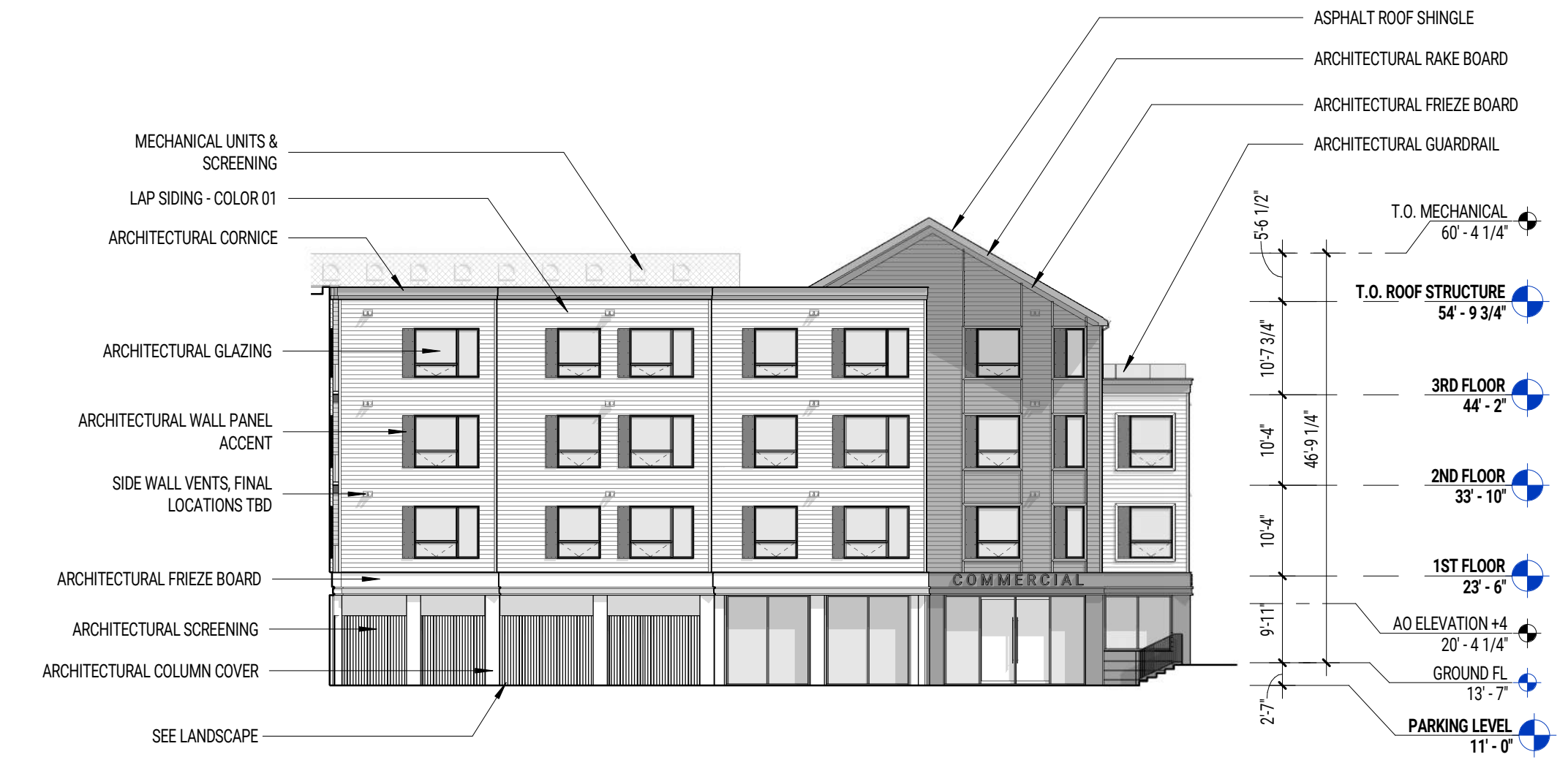
7 COURTYARD 02 - SAWTOOTH BAYS 02 SCALE: 1/16" = 1'-0"
