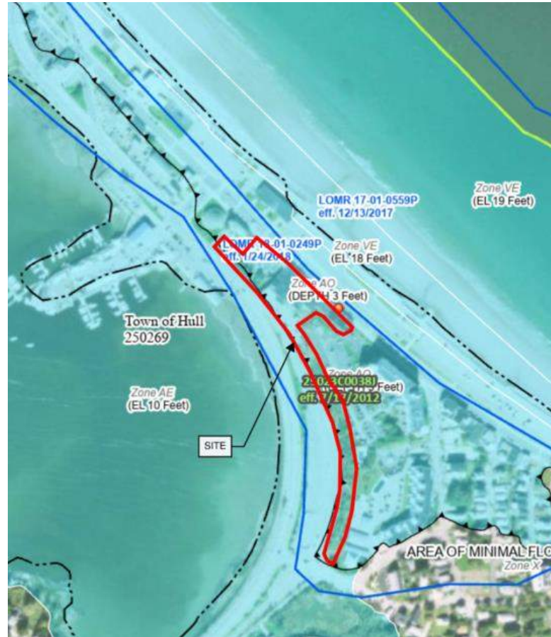
Land Subject to Coastal Storm Flowage (LSCSF)
