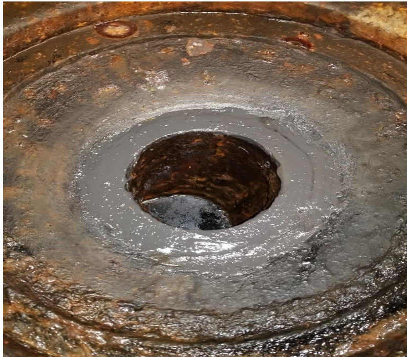
Built-up casing wear ring for influent pump #1 with ceramic coating
