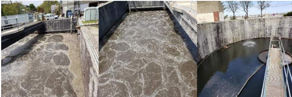
Aeration tank #1- moderate foam
