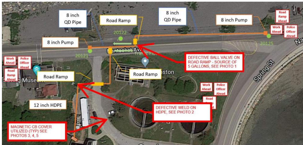
6/2/20 spill at the wastewater plant due to defective pipe weld
