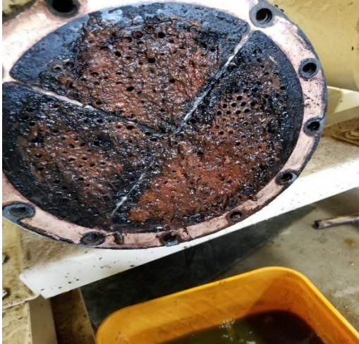
Gen #1 internal blockage & corroded tubes
