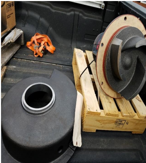
New volute and repaired rotating assembly
