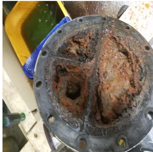
Corroded end cap of heat exchanger
