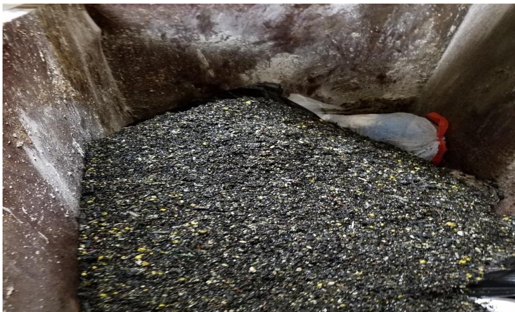
Grit deposited from classifier into rag/screening cart
