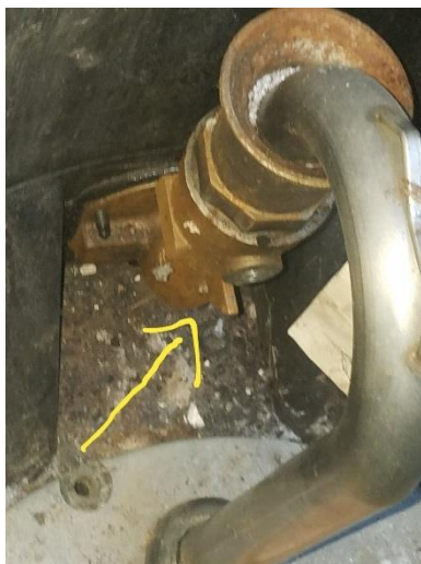
61 Wyola – failed discharge isolation valve [frozen]
