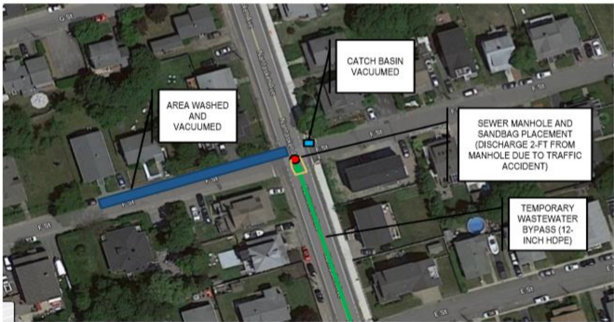
FIGURE 1: DIAGRAM OF SANITARY SEWER OVERFLOW ON 12/9/2019 DUE TO TRAFFIC ACCIDENT – HULL MA
