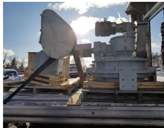
Thickener drive unit on left tipped on broken pallet
