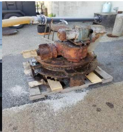
Old gear box removed
