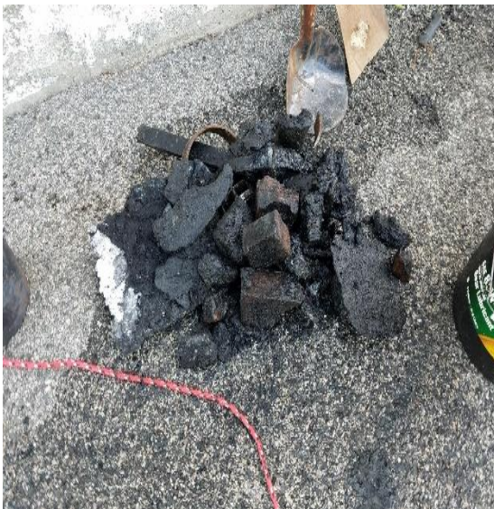
Debris collected from bottom of the wet well
