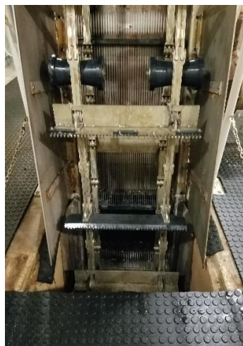
Flex rake bar screen
