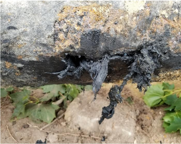
Corroded/rotted force main pipe segment
