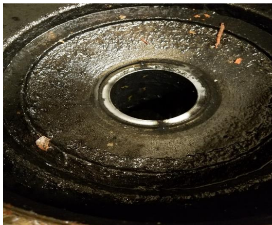
pump volute – wear on internal bowl component
