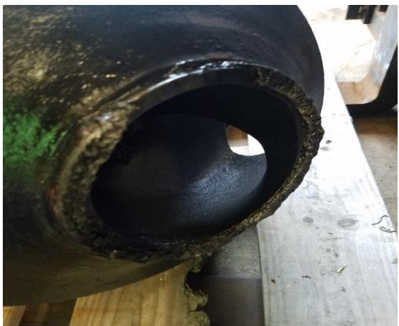
Worn impeller wear ring [rotating element]
