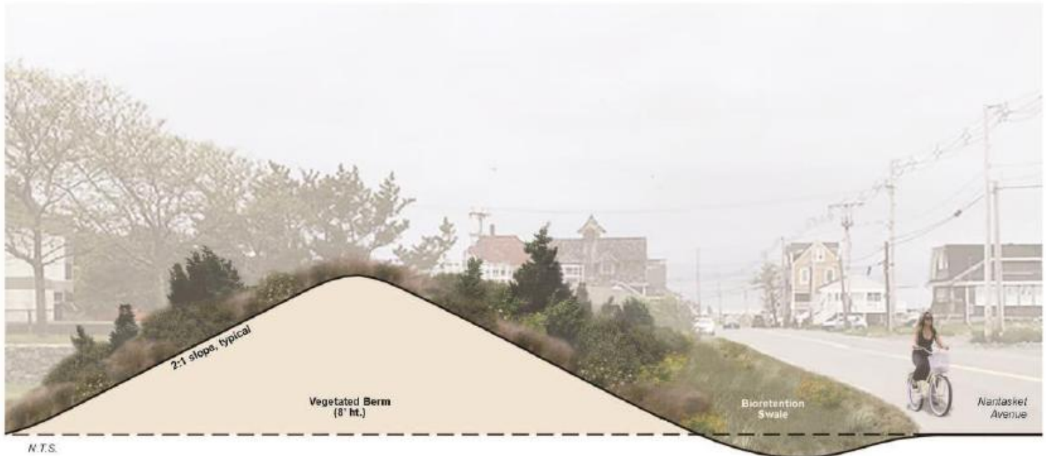
Photo-rendering of the proposed berm to serve as flood protection at the WWTF, funded by Coastal Zone Management (CZM).
