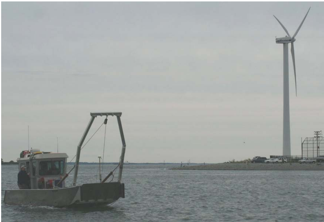
Photograph 2 R/V Lophius collected bathymetric, side scan sonar, and magnetic data
