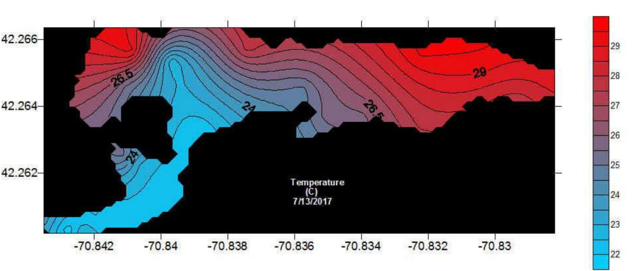
**Figure 3**. Spatial distribution of Temperature (°C) in the surface water of Straits Pond, Cooler waters indicated in blue.
