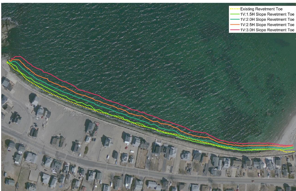
Figure 4.9. Seaward extent of revetment toe for a 25 ft MLW revetment with 1.5, 1:2, 1:2.5 and 1:3 revetment slope. Extents are representative for Option 7.
