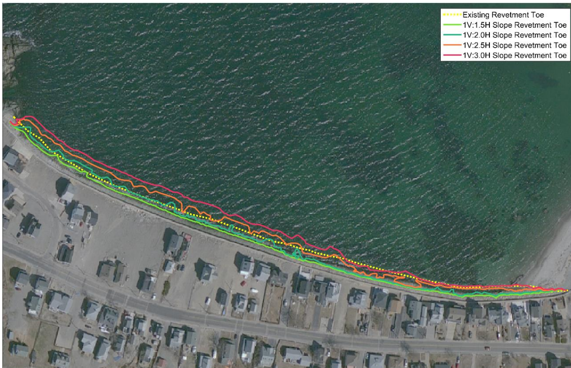
Figure 4.7. Seaward extent of revetment toe for a 17 ft MLW revetment with 1.5, 1:2, 1:2.5 and 1:3 revetment slope. Extents are representative for Option 1, 2 and 3.
