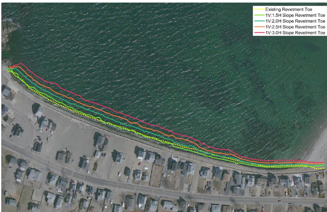
Figure 4.8. Seaward extent of revetment toe for a 23 ft MLW revetment with 1.5, 1:2, 1:2.5 and 1:3 revetment slope. Extents are representative for Option 4, 5 and 6.
