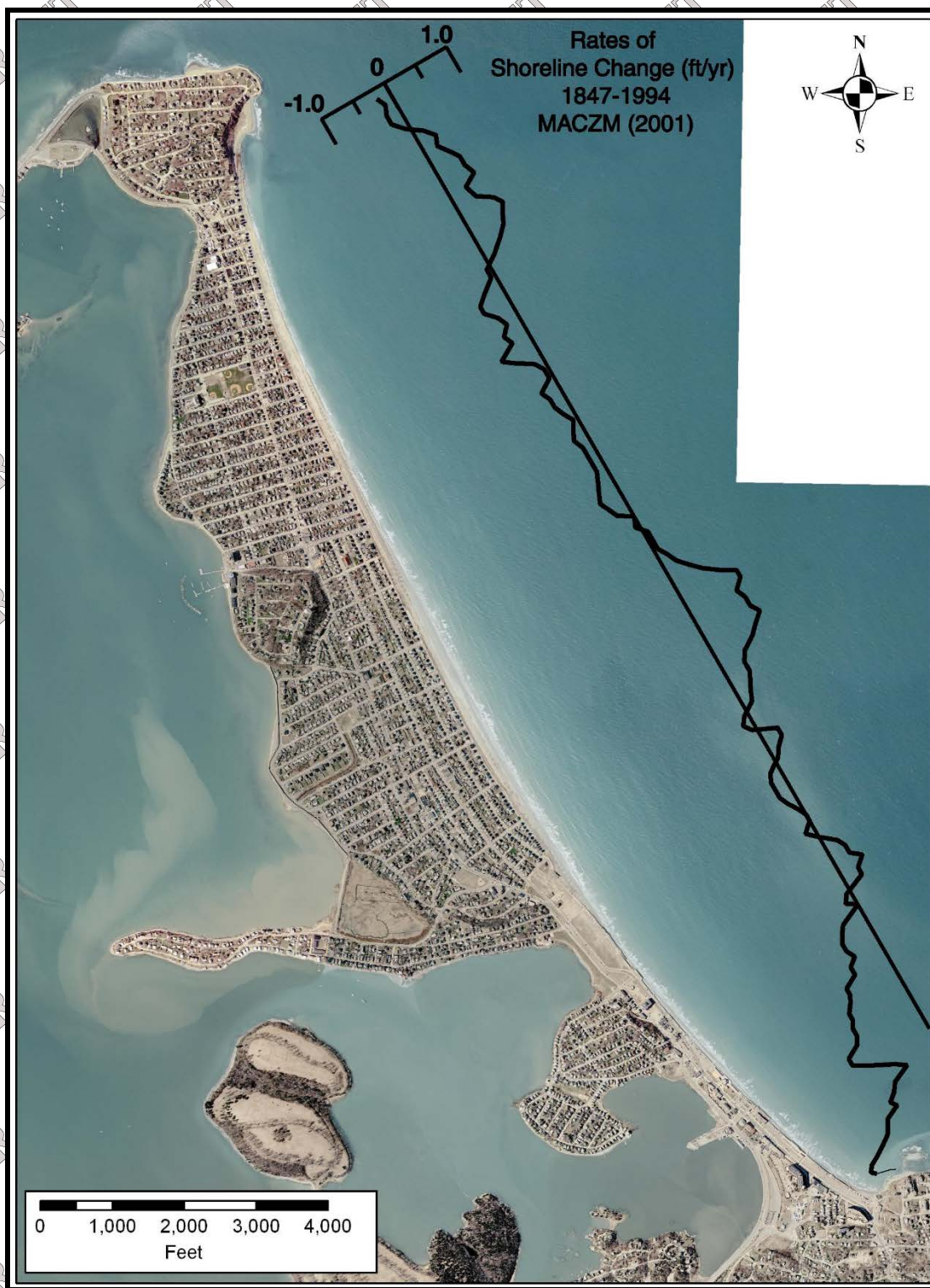
Figure 3-1. Rates of historic shoreline change between 1847 and 1994 as determined by Massachusetts Coastal Zone Management (2001).
