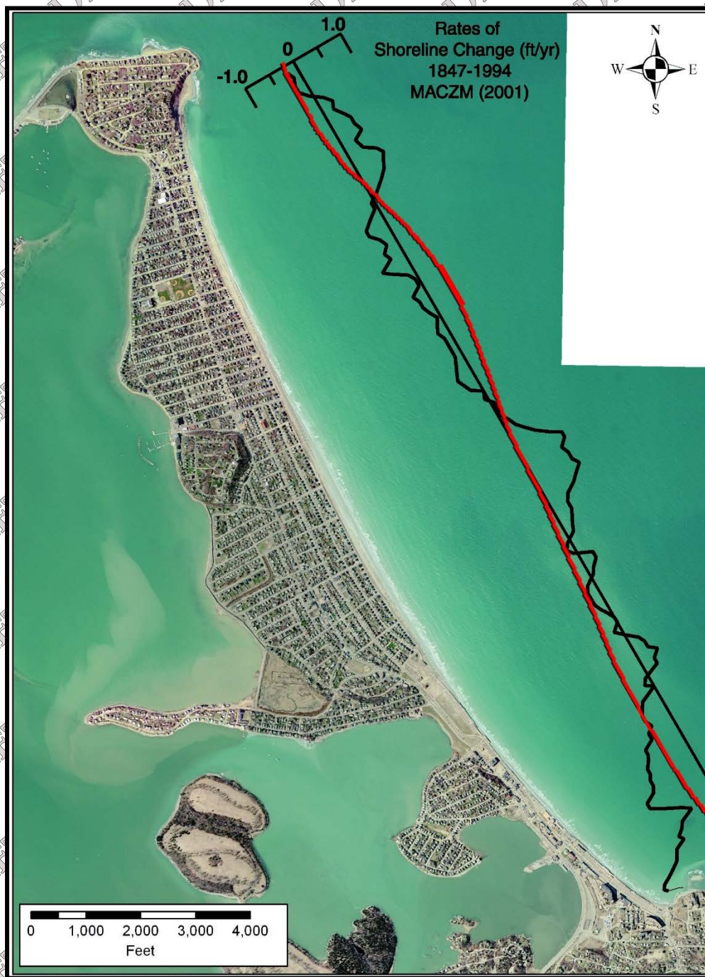
Figure 5-6. Sediment transport flux from modeling results (red line) compared to historic rates of shoreline change (ft/yr black line).
