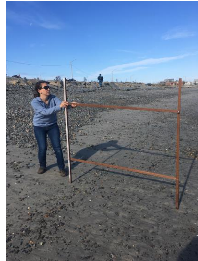
Beach profiling using a modified Emery-rod method for determining beach elevation along a transect near Phipps St.
